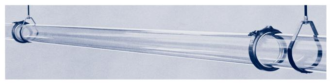
KIMAX Glass Pipe requires less hangers than polypropylene and high silicon iron pipes - only one hanger every 8 to 10 feet.
